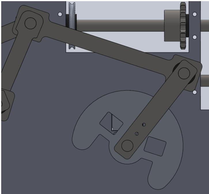
Figure 20: CAD model of the crank rocker
