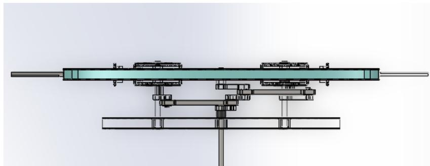
Figure 50: **Outriggers top view connected to the main frame through the shaft (displayed in the bottom).**
