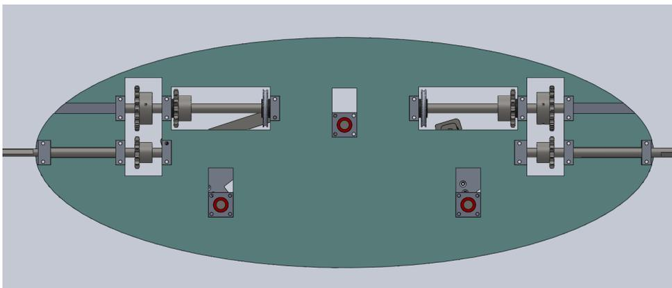
Figure 22: Bearing blocks embedded in the keel
