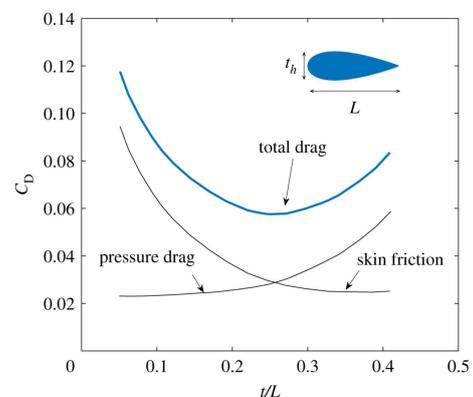
Figure 1: **Contribution of pressure drag and skin friction to the total drag.** The  $C_D$  data were obtained by dividing drag-per-unit-length data by  $1/2\rho U^2 t_h$  (Godoy-Diana and Thiria, 2018).
