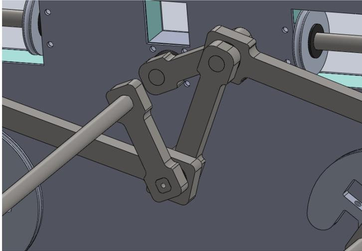
Figure 19: CAD model of the crankshaft system
