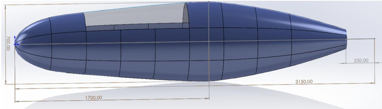
Figure 3: **Design of the Hull.** The hull consists of even parts and a big hatch for the pilot. The safety-buoy at the end of the submarine is not included in the hull design.
