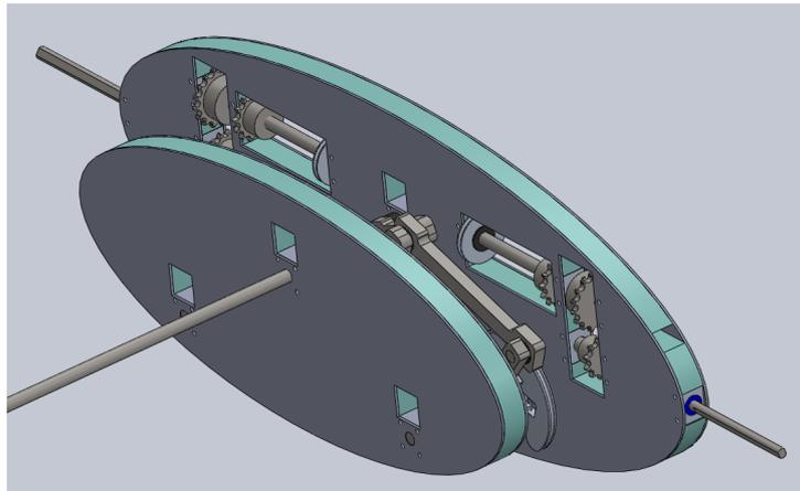
Figure 18: CAD model of the full transmission system in the outrigger. The MirageDrive fins will be attached in pairs to the protruding shafts in the top left and bottom right corner.
