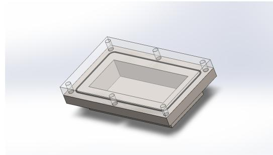
Figure 37: Sealed box holds two motor drivers and Arduino Nano
