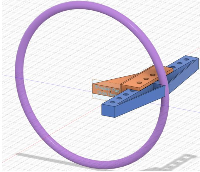
Figure 42: **Ideation of the shoulder pad setup.** Note that the pad itself is not included, rather only a proposition of how it could attach to the frame.
