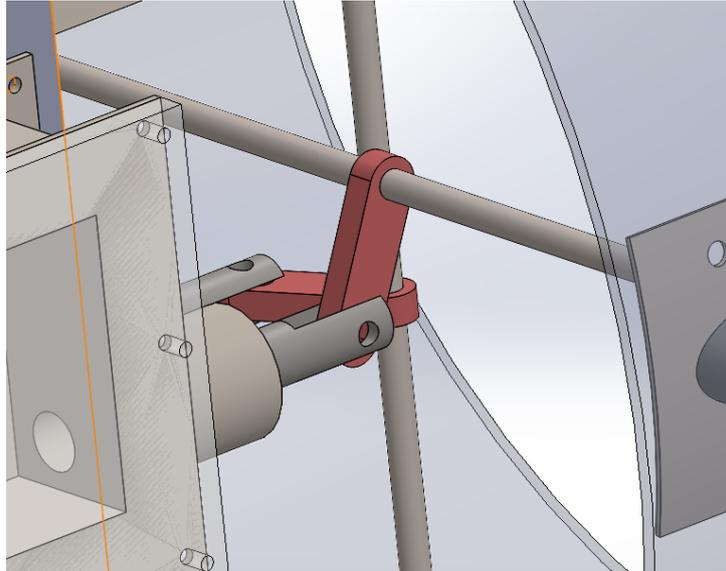
Figure 29: **Simple crank slider mechanism.** An aluminium link is attached between the linear actuator and the elevator shaft.
