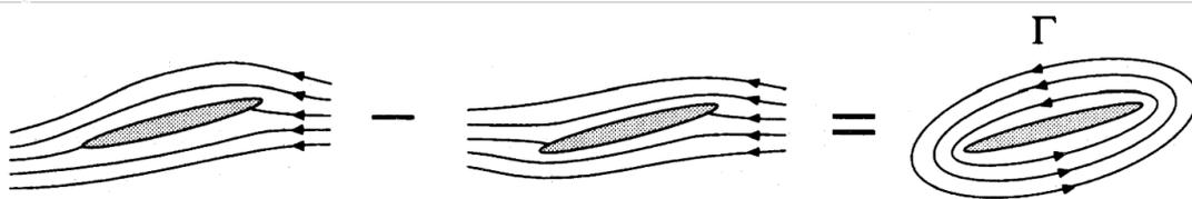
Figure 11: **Steady-state Theory of Lift.** A flow over a hydrofoil with an angle of attack shows an asymmetrical velocity field (left). If the theoretical background symmetrical field (middle) is subtracted, a net circulation is obtained (right) that induces the differences in velocities on both sides of the hydrofoil. The velocity on the upper side is higher than on the lower. Modified from (Dickinson, 1996).
