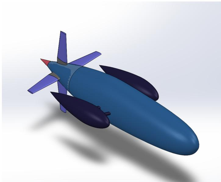
Figure 25: *Cygnus IV* in modelling phase. Cross plane rudders are attached at the end.
