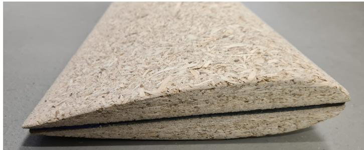
Figure F: **Arrangement of the Rudders.** The two wooden halves of the rudders show an aluminium plate between them for additional stability during usage.
