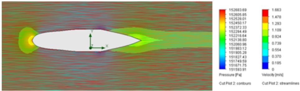
Figure C: **Cut Plot Velocity Pressure** . Modified from HSRW submarine team (2018)
