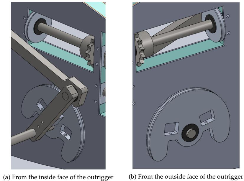
Figure 21: CAD models of the pulley system, chain and wires not shown
