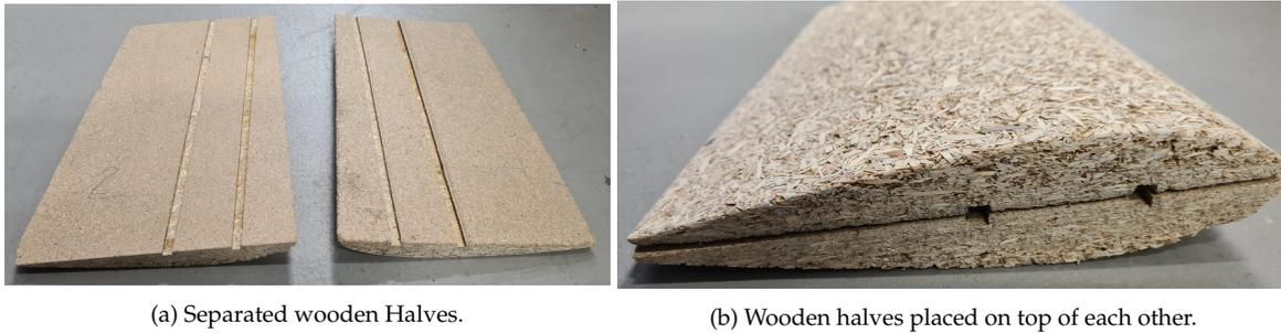
Figure G: The two wooden halves (a) of the stabiliser fins show two parallel grooves on the symmetry plane. In (b) both fins are placed on top of each other
