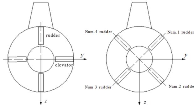
Figure 26: **Cross plane rudders to X-Plane.** For the rudders Cross plane is used on *Cygnus IV*.
