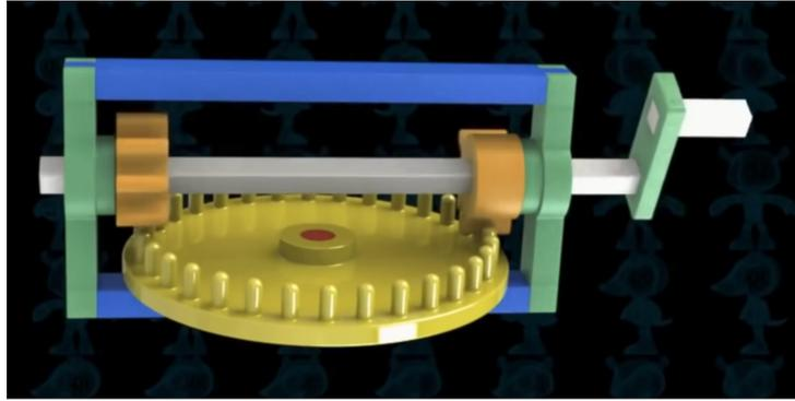
Figure 14: Concept drawing for a half bevel system. (Franco Fonnese, 2018)
