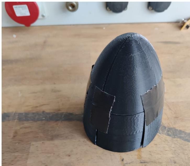
Figure 43: 3d printed scale model of the hull
