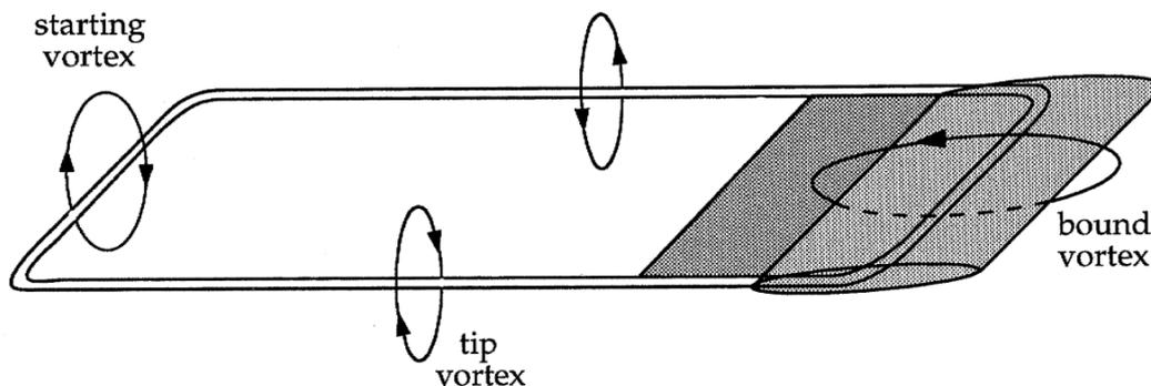
Figure 12: **Lift by Induced Vortices.** Lift is generated by the wake momentum. The starting vortex, the tip vortices and the bound vortex build a closed loop with circulation of zero in total. Modified from (Dickinson, 1996).
