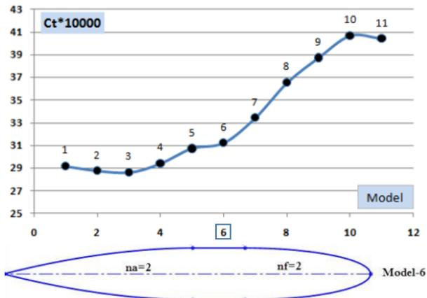
Figure 2: Total resistance coefficient for multiple Models (based on wetted surface area). Model six was chosen as design basis. Modified after Moonesun et al. (2015)
