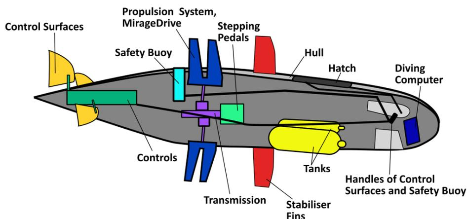
Figure H: **General Arrangement of *Rivershark Mod III***. Layout of *Rivershark Mod III* with the position new safety buoy and stabiliser fins.
