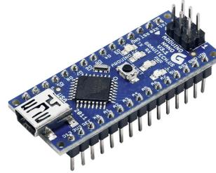
Figure 32: Arduino Nano used for the electronic circuit
