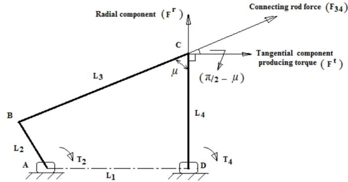
Figure 16: Simplified crank rocker system (Mohammed et al., 2006)
