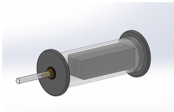
Figure 38: Battery Box that fits two LI-PO batteries inside
