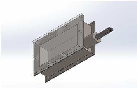
Figure 36: Linear actuator sealing box
