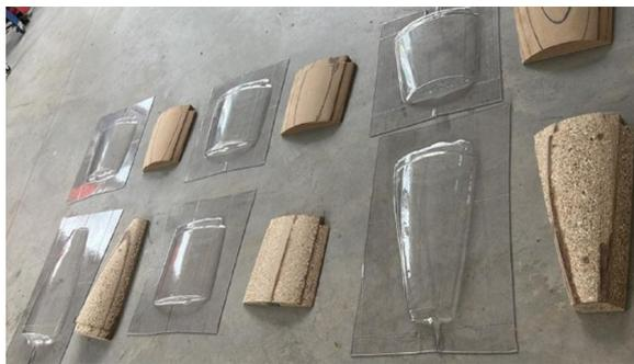
Figure 5: **Positive moulds and vacuum formed PET-G parts** . Each hull section was formed by a different mould.
