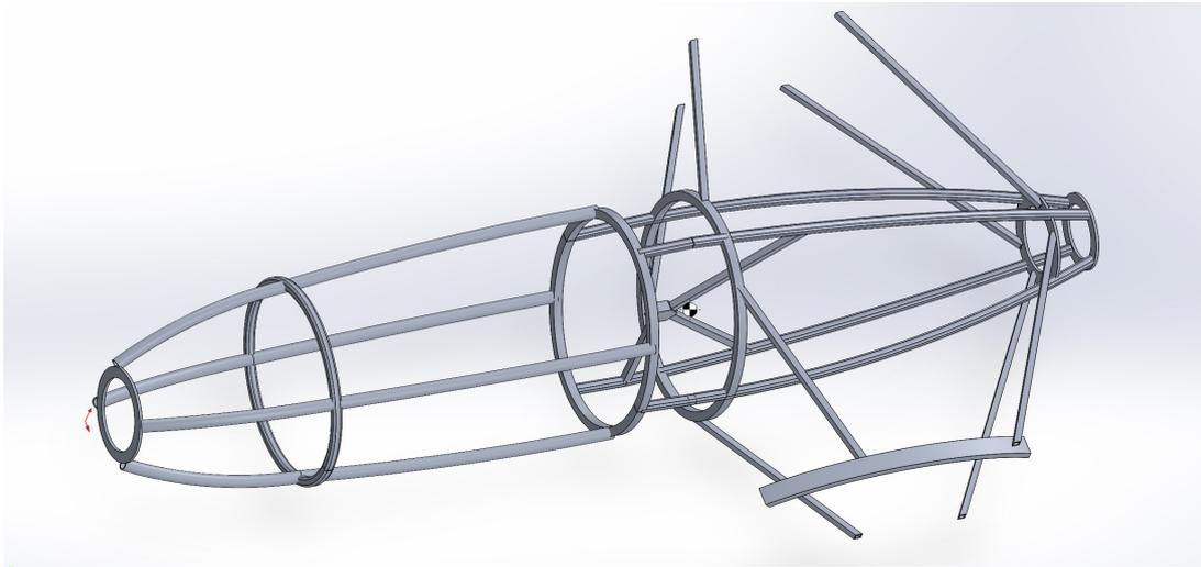
Figure 7: **Design of the Frame.** Frame is consisting of five ellipses connected with several straight tubes. In the back the tubes are connected to the outriggers.
