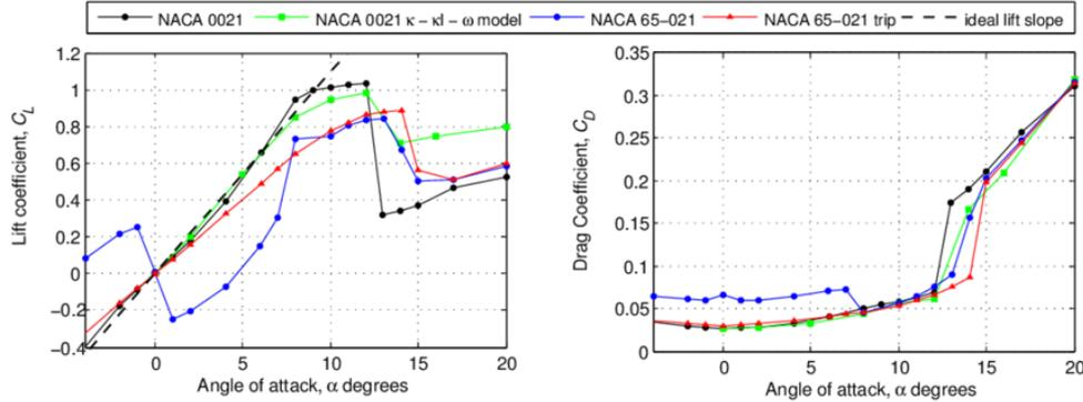
Figure 28: lift Coefficient values compared to angle of attack. Modified from Hansen et al. (2014).
